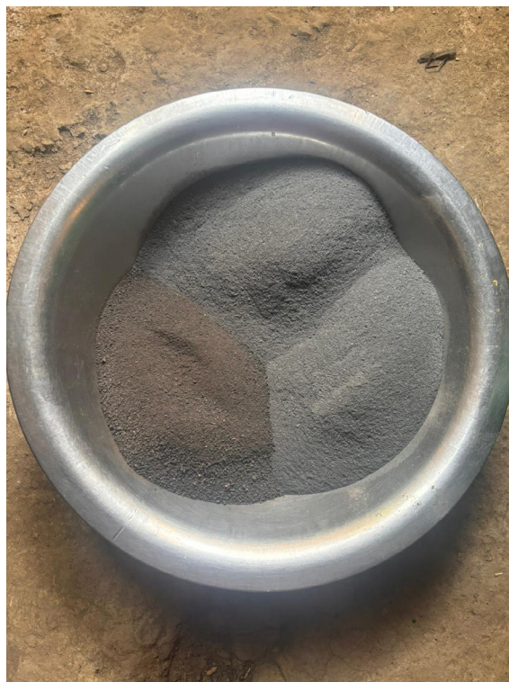
Figure 7. Mixing the proper ratio of clay is the most important part of pottery-making. The right amount of clay is needed, which consists of one sack of tsükro (grog) and two sacks of dried clay ( ranyuo ) kept in a bowl to make a dough. Photo credit: Author
