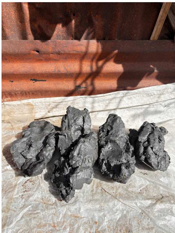
Figure 4. After digging up the fresh clay, the next critical step was to sun-dry it for a week or longer, depending on the weather conditions. When the clay is completely dried, it hardens and is ready to be pounded. Photo credit: Author
