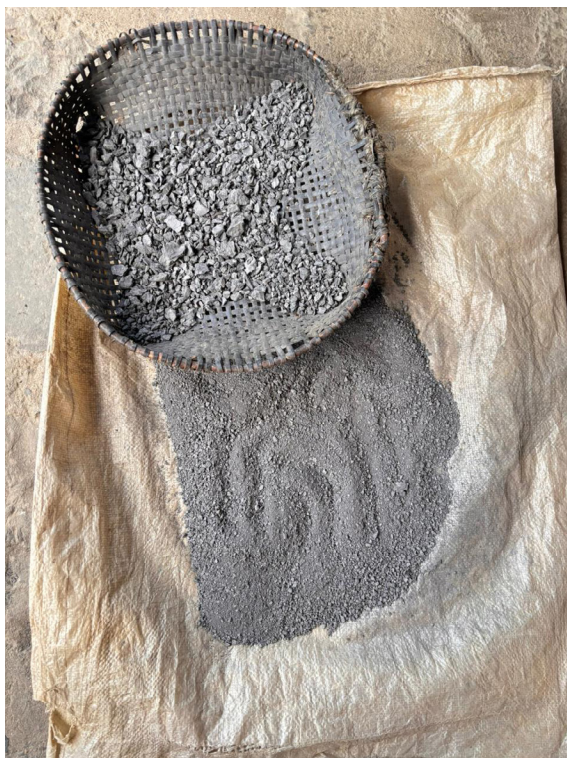
Figure 5. Sun-dried clay was pounded in a wooden mortar with the help of a pestle and was sieved with a bamboo net to remove coarse, unwanted particles and make a refined powder. The more refined the clay powder, the better it will be while molding and shaping the structure. Photo credit: Author
