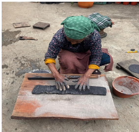
Figure 11. Ash was applied to the wooden board so that the clay would not get stuck on the board while working, and a wooden spatula, paddle, and beater were used to beat the clay to form a uniform texture. Photo credit: Author
