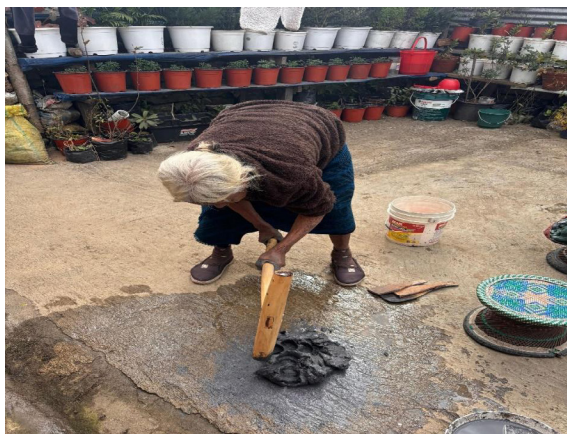
Figure 9. Clay mixed with water by bare hands was again pounded by a wooden beater ( mavü ) to properly mix the material and make it sticky and soft. When the process is done, it will be more pliable and elastic for shaping and molding into the pot the potter desires. Photo credit: Author
