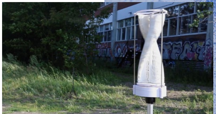
Figure 7 Air Turbine gathering wind speed data and particulate matter.
